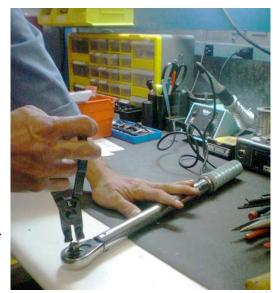
torque wrenches should be serviced in line with manufacturers recommendations or no longer than 100,000 cycles, or when a visual inspection reveals old or dry grease, parts that show signs of excessive wear, loose or unstable components.
